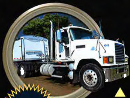
2009 Mack Model CHU613 Tandem Axle Conventional Day Cab Truck Tractor VIN# 1M2AND7C19N004401, Mack MP8- 445E Turbo Diesel Engine (445 HP), Mack Maxitorque 18-Speed, 175,306 Miles.
